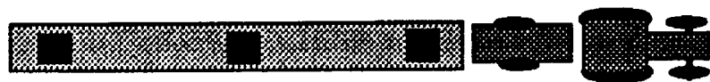
Figure 2. Three or more plastic sheets placed in the path of the manure spreader can be used to estimate application rate.
